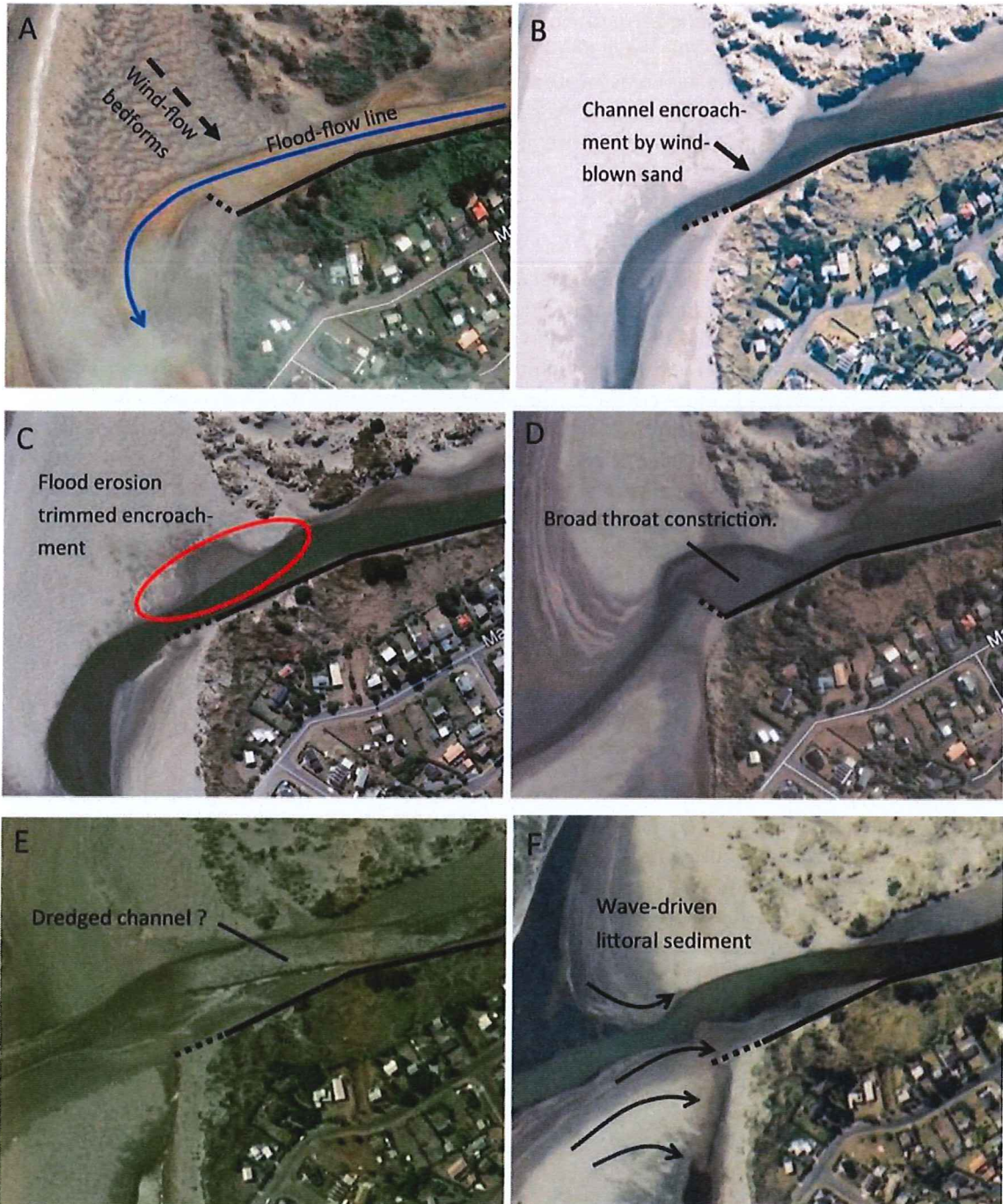
Figure 11: Configurations associated with throat constriction - see text for explanations. The black line defines the rock-lined southern embankment and the dashed black line marks the various entrance groyne. The bend mid-way along the southern embankment (black line) results in an approach channel misalignment with the original entrance groyne (dashed line in Figures B, C, E and F). Note the (apparently) dredged channel in E is more closely aligned with the upstream section of the marked southern embankment.
