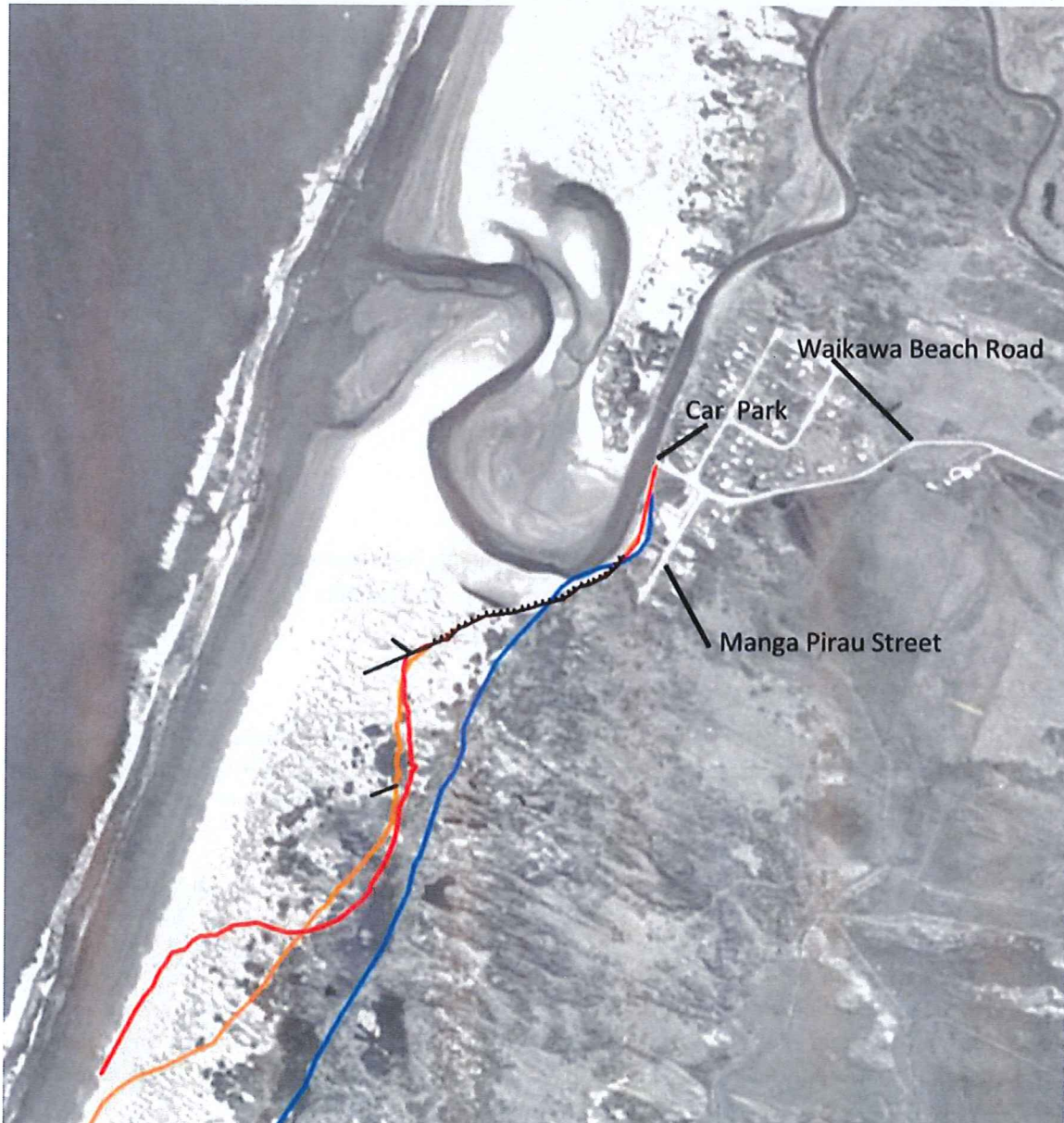
Figure 5: Typical post 1945-diversion response morphology on the 1968 aerial photo with the river meandering northward. The 1942 shoreline is marked purple, 1993 by orange and current 2018 by red. Structures are marked black as in Figure 4.
