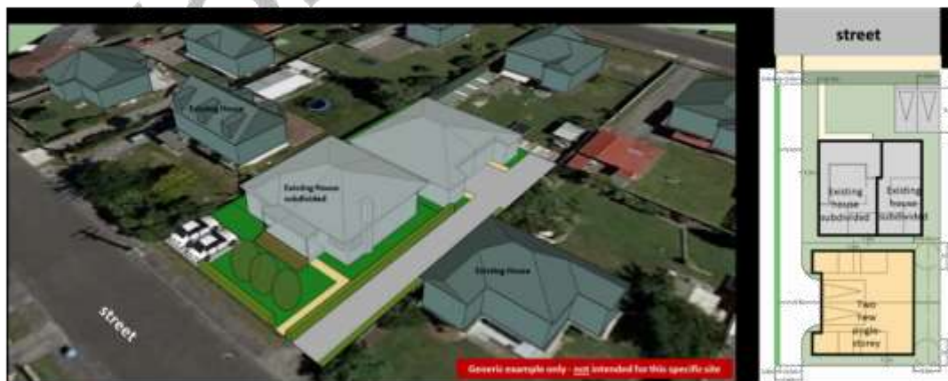
Figure 3-10. Two single-storey, two-bedroom dwellings behind the existing house subdivided into two apartments.
