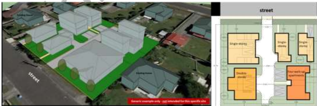
Figure 3-13. Four single-storey, two-bedroom dwellings, two double-storey, three-bedroom dwellings, and four two-bedroom walk-up apartments.
